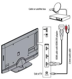
Connect a 3.5mm audio cable (not provided) to the PC/DVI AUDIO IN jack on the side of your TV and to the **AUDIO OUT** jacks on the cable or satellite box.
